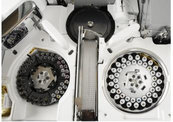
Indiko Plus has a sample disk for up to 108 samples : 9- or 18-position sample racks, max 6 racks. Reagent disk in Indiko Plus has positions for 42 reagents.
