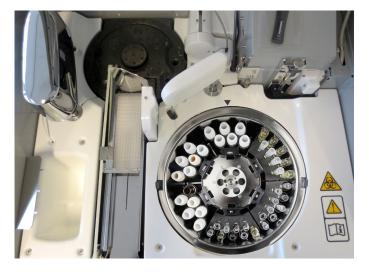
Indiko includes combined sample and reagent disk for max 6 racks: 9-or 18-position sample racks and 6-position reagent racks.
