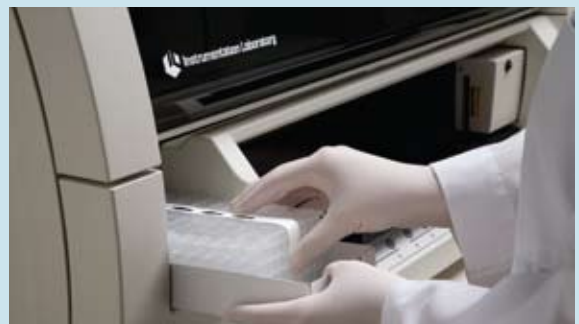
Continuous cuvette loading allows for uninterrupted operation.
