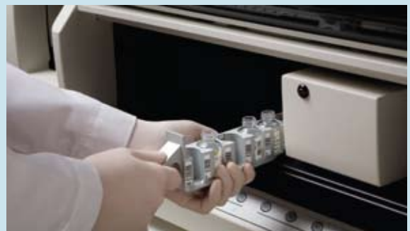
Real-time reagent management with onboard barcode reader.
