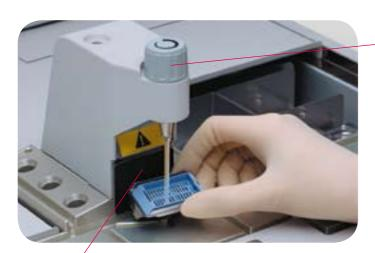
Finger touch plate and optional foot switch control the paraffin flow The Tissue-Tek® TEC™ Tissue Embedding Console System has always maintained an outstanding record of quality and reliability.
