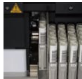
The rack at the left end is loaded into the analyzer, and the cup sensor recognizes the samples. The barcode reader then reads the sample IDs.
