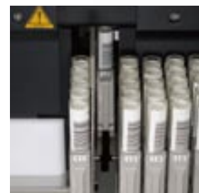
Racks for which sampling has been completed are pushed out of the analyzer and moved to the left end of the sampler.
